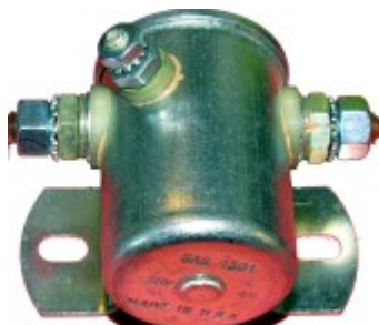
*36V* "SPECIAL" SWITCH ACTIVATES WHEN GROUNDING THE SMALL 10/32 POST REPLACES, SAS-4304 "WMS" PART # 15-350
