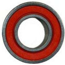
“SEALED” BALL BEARING WITH A 6-202-4 “OD” AND A 6-203-4 “ID” “WMS” PART NUMBER WBB-103 ID 17 mm < OD 35 mm Width 10 mm
