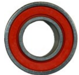
“SEALED” BALL BEARING FOR WINCH MOTOR W-9133 & W-9143 DE “WMS” PART NUMBER WBB-6004 ID 20 mm < OD 42 mm Width 12 mm
