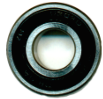
“SEALED” BALL BEARING REPLACES NUMBERS 202, 6-202-2, 6-202-4 “WMS” PART NUMBER WBB-202 ID 15 mm < OD 35 mm Width 11 mm
