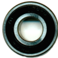
“SEALED” BALL BEARING WITH A 6-202-4 “OD” AND A 5/8” “ID” “WMS” PART NUMBER WBB-20210 ID 15.88 mm < OD 35 mm Width 11 mm
