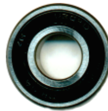
“SEALED” BALL BEARING WITH A 6-203-4 “OD” AND A 5/8” “ID” “WMS” PART NUMBER WBB-20310 ID 15.88 mm < OD 40 mm Width 12 mm
