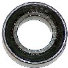
“SEALED” BALL BEARING REPLACES NUMBERS 6902, 6-902-4 “WMS” PART NUMBER WBB-8815DEB ID 15 mm < OD 28 mm Width 7 mm
