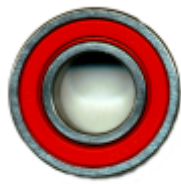
“SEALED” BALL BEARING WITH A 6-201-4 “OD” AND A 6-202-4 “ID” “WMS” PART NUMBER WBB-212 ID 15 mm < OD 32 mm Width 9 mm
