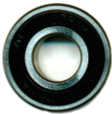
“SEALED” BALL BEARING REPLACES NUMBERS 203, 6-203-2, 6-203-4 “WMS” PART NUMBER WBB-203 ID 17 mm < OD 40 mm Width 12 mm
