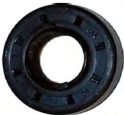
SHAFT SEAL FOR THE 4.8" DIAMETER BUYERS AND MEYER STYLE SPREADER MOTOR NUMBERS W-8805 AND W-8858 PART # WSS-8805 O.D. IS 1.190 < I.D. IS 0.550
