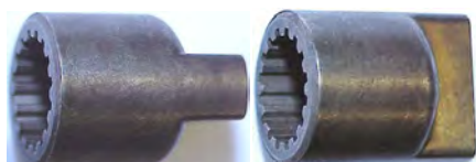
# J3-1001-14 ( 16 SPLINE W/TANG ) 0.764"/ 19.40mm LONG TANG IS 0.250"/ 6.35mm WIDE
