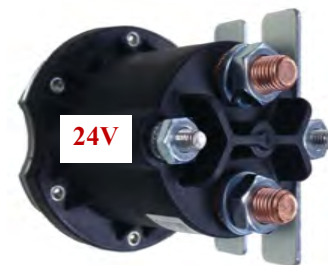
*24V* CONT/DUTY 4 POST SW. REP. 684-2451-022, 684-2451-240 “WMS” NUMBER, WS-937 switch has standard bracket with 0.275 mount/slots that are approximately 1” forward from rear plate area. ( FLAT MOUNT W/INS GROUND )
