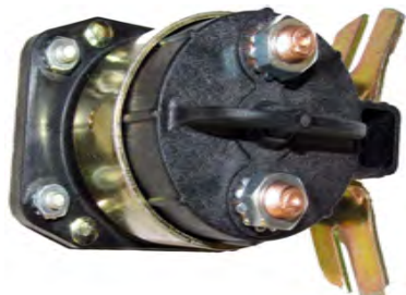
*12V* CONTINUOUS DUTY INS/GRD 4 POST SWITCH REP. 586-902, 114-1211-010, 114-1211-020 “WMS” NUMBER, WS-812C Surge Amps 600 < Continuous Amps 200 Motors, W5144, MBR5102N, W5001, W8163 ( The switch has a curved mount base )
