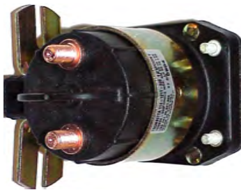
*12V* CONTINUOUS DUTY INS/GRD 4 POST SWITCH REP. 586-902, 114-1211-010, 114-1211-020 “WMS” NUMBER, WS-812F Surge Amps 600 < Continuous Amps 200 Motors, C561350X8081, X7642, W8163 ( The switch has a flat mount base )
